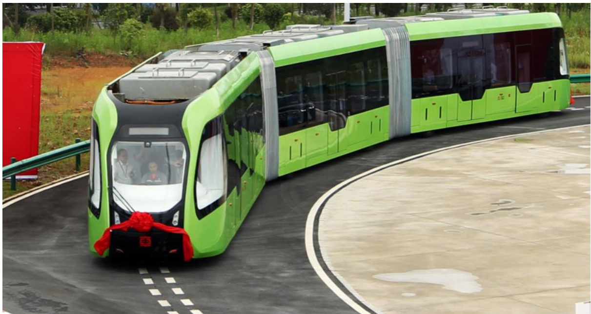
Figure 1-4: "Trackless tram" in Zhuzhou, China. Self-driving vehicles, with rubber wheels, using sensor technology to follow markings painted on the streets
