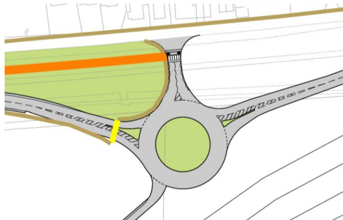
Figure 24 – A parallel crossing with increased stacking space on the northern arm of the London Road Roundabout, possible by reducing its ICD
